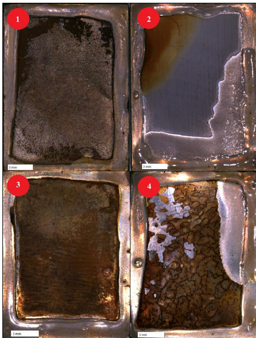
Figure 3 - Comparison between blank and lower rate coating (2 - Coating with TEOS only; 4 - Coating with TEOS and Zinc)
